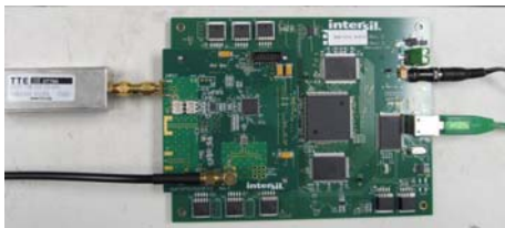
FIGURE 3. DAUGHTERBOARD WITH KMB MOTHERBOARD
